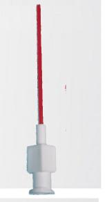
Teflon lined tips for dispensing Cyanoacrylate adhesives. PTFE Teflon tube resists clogging. 0.50" or 1.0" long. Polypro hub material to stainless steel tube with Teflon crimped insert. Double helix threaded luer lock colour coded hub. Boxes of 50, 500 or 1000.
