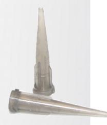
The TE needle series consist of a stainless-steel shaft with a double helix polypropylene hub. This premier line of dispensing needles is burr-free, and electro-polished shaft for unobstructed and consistent material flow. They are silicone and chloride free. For most viscosity fluids and adhesives and safe for use to 100 psi. Supplied in packs of 50, 500 or 1000 tips.
